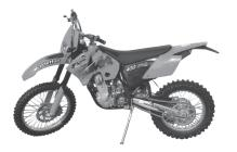
**Class I** off-highway vehicle has two low pressure tires, a saddle seat designed to be straddled by the operator, and it is steered by the use of handlebars.
